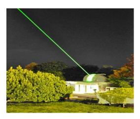
The project Rayleigh Doppler Lidar (RDL) uses a high energy laser with 30W power @532nm and 50Hz repetition rate to get atmospheric backscattering from molecules and particles. A 750mm telescope in Newtonian configuration is used to collect the signal from athe atmosphere and a Fabry Perot Interferometer as frequency discriminator is employed to get the radial winds. A few photographs of Pic 1 and 2 of the system are shown. The Project is completed, and Zonal and Meridional
